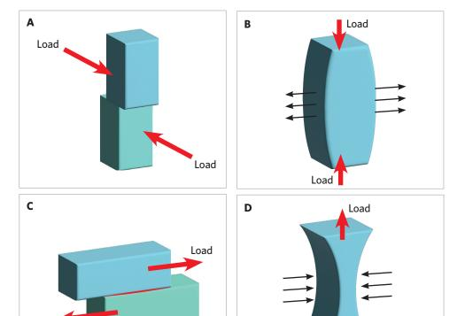
Figure 1. Types of force: (a) shear, (b) compression, (c) frictional, and (d) tensile force/strain (Baker and Osman, 2016).
